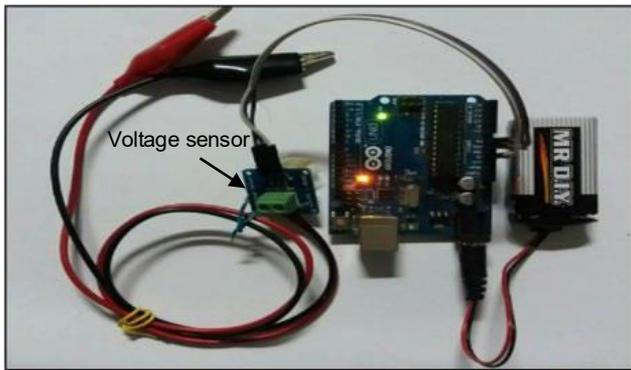
Fig. 6: Battery voltage measurement using voltage sensor circuit
